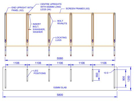
ASSEMBLE THE SHELTER INCLUDING THE SEATING. PLACE IN THE REQUIRED POSITION. MARK THE ANCHOR HOLE POSITIONS. MOVE THE SHELTER TO DRILL THE HOLES. REPOSITION THE SHELTER AND INSERT THE SCREWS.
