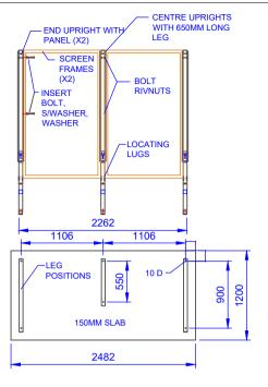
ASSEMBLE THE SHELTER INCLUDING THE SEATING. PLACE IN THE REQUIRED POSITION. MARK THE ANCHOR HOLE POSITIONS. MOVE THE SHELTER TO DRILL THE HOLES. REPOSITION THE SHELTER AND INSERT THE SCREWS.
