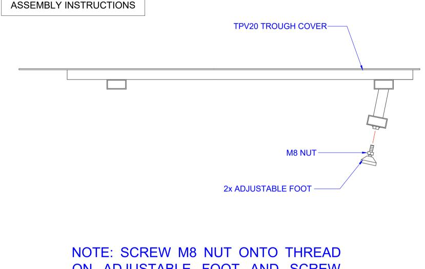
NOTE: SCREW M8 NUT ONTO THREAD ON ADJUSTABLE FOOT AND SCREW ADJUSTABLE FOOT ONTO TROUGH COVER. USE LOOSE NUT TO LOCK ADJUSTABLE FOOT IN PLACE WHEN CORRECT HEIGHT HAS BEEN REACHED.
