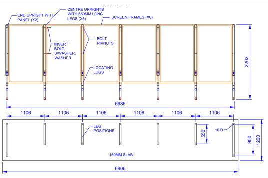
ASSEMBLE THE SHELTER INCLUDING THE SEATING. PLACE IN THE REQUIRED POSITION. MARK THE ANCHOR HOLE POSITIONS. MOVE THE SHELTER TO DRILL THE HOLES. REPOSITION THE SHELTER AND INSERT THE SCREWS.
