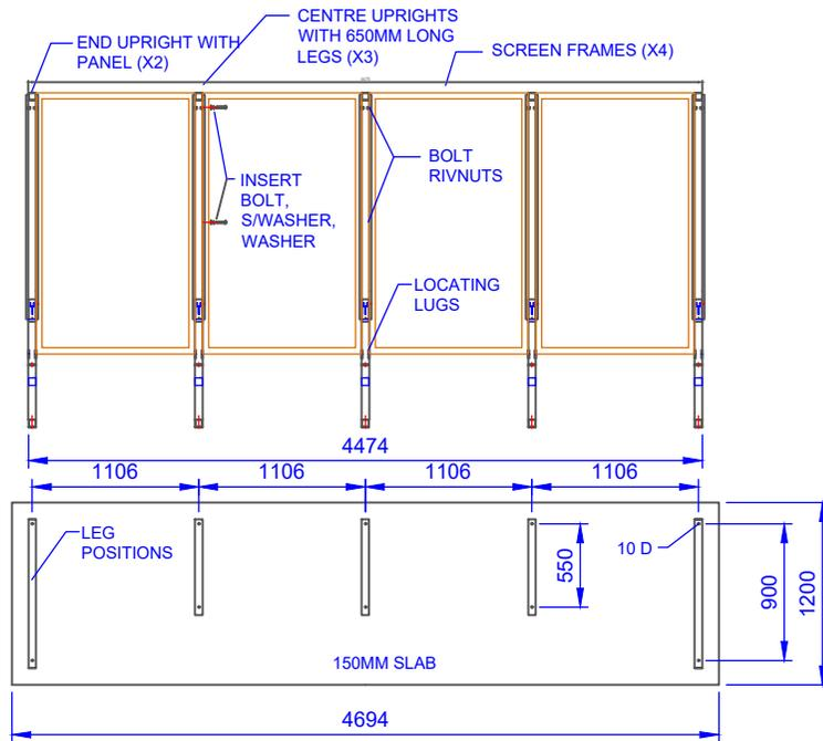
ASSEMBLE THE SHELTER INCLUDING THE SEATING. PLACE IN THE REQUIRED POSITION. MARK THE ANCHOR HOLE POSITIONS. MOVE THE SHELTER TO DRILL THE HOLES. REPOSITION THE SHELTER AND INSERT THE SCREWS.
