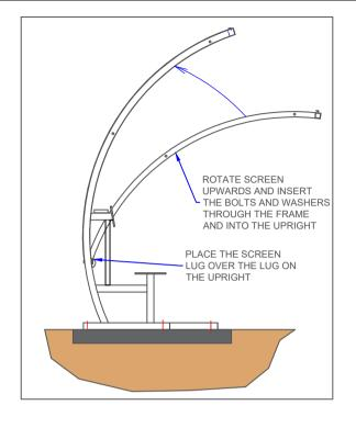
ASSEMBLE THE SHELTER INCLUDING THE SEATING. PLACE IN THE REQUIRED POSITION. MARK THE ANCHOE HOLE POSITIONS. MOVE THE SHELTER TO DRILL THE HOLES. REPOSITION THE SHELTER AND INSERT THE SCREWS.
