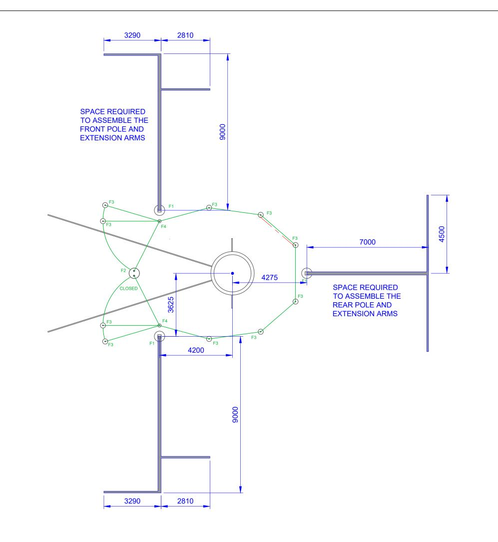
TITLE: THOR 9 HAMMER CAGE SPACE REQUIRED AROUND THE CAGE TO ASSEMBLE DRAWING NUMBER: CHECKED BY: THOR 9 DESIGNED BY: DRAWN BY: UMESH TREVOR ACOT.: 07/11/2023 TOLERANCE:  $0.0 \pm 1.0$   $0.0^{\circ} \pm 1^{\circ}$  SCALE:  $0.00 \pm 0.5$   $0.00^{\circ} \pm 0.5^{\circ}$   $0.000 \pm 0.2$ SYSTEM: **A3** ♦ 母
